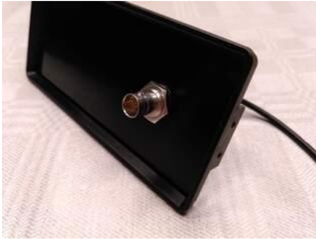
Figure 3. 75 \Omega BNC connector installed
