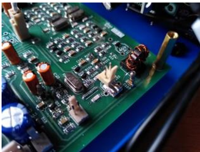
Figure 10. CW carrier connector mod
