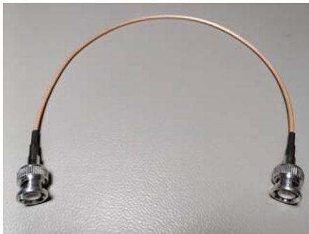
Figure 7. RG316 patch cable (crimping practice)
