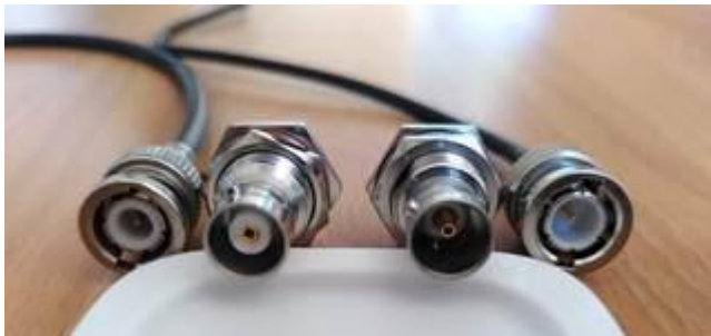
Figure 4. 50 \Omega BNCs (left) vs 75 \Omega BNCs (right)
