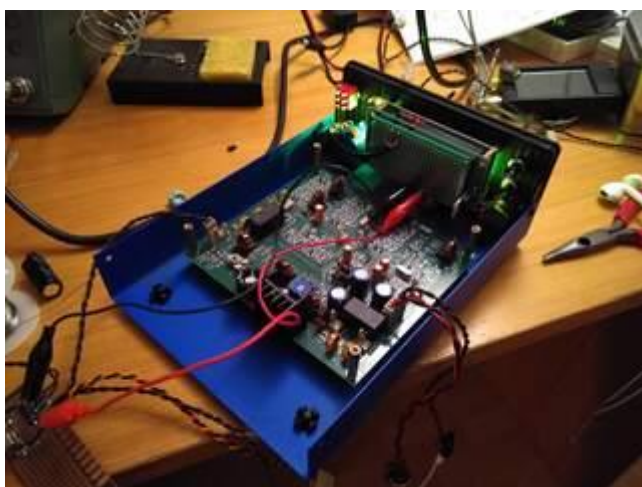
Figure 9. Testing (the lack of) extra voltage regulator capacitors on the Raduino
